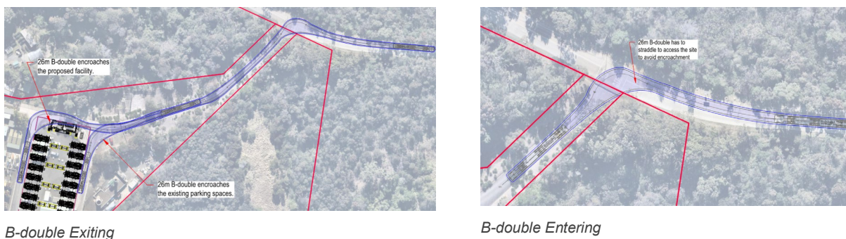
Figure 4.7 Swept path analysis Insets (B-double, 26 metres)
